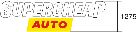
SIGN 7: 3D CORPORATE LOGO (FLOOD LIT) Overall Size: 4338 w x 1275mm h Supercheap Letters: 4338 w x 689mm h Yellow with Auto: 1906 w x 577mm h 3D Logo fixed directly to wall
