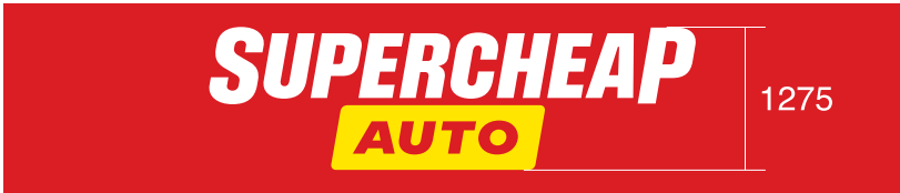
SIGN 1: 3D CORPORATE LOGO (FLOOD LIT) Panel Size: 8000 w x 1700mm h Overall Size: 4338 w x 1275mm h Supercheap Letters: 4338 w x 689mm h Yellow with Auto: 1906 w x 577mm h Aluminium frame and ACM cladding over existing lightbox with 3D corporate logo
