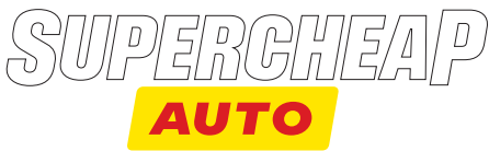
SIGN 13: 3D CORPORATE LOGO Overall Size: 4338 w x 1275mm h Supercheap Letters: 4338 w x 689mm h Yellow with Auto: 1906 w x 577mm h 3D Logo fixed directly to wall
