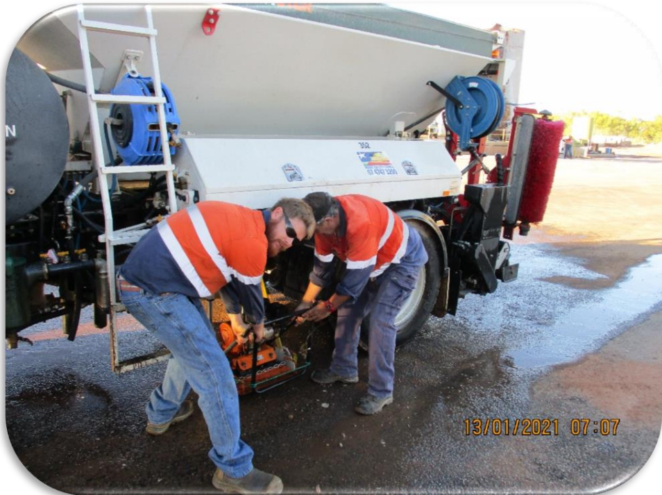
Figure 2: Works conducted on the Oz Road Bitumen Patching Machine to retrofit a plate lifter, improving safe operation for the operator.
