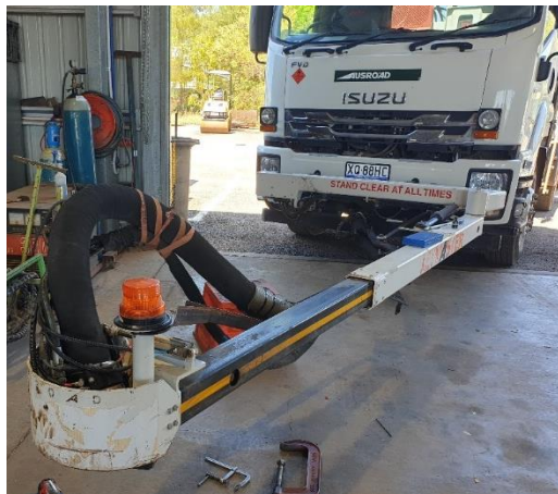
Figure 2: Repairs to Jet Patcher arm to improve on strength and structure.
